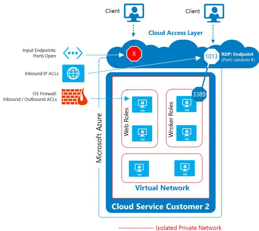
Figure 6. Topology of Azure Cloud Services Virtual Networks.
