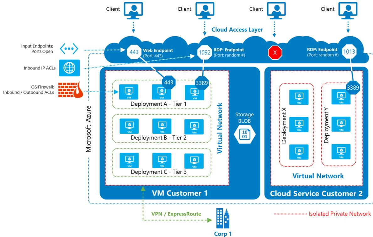
**Figure 1. An example of isolated multi-tier IaaS applications hosted within Azure.**
