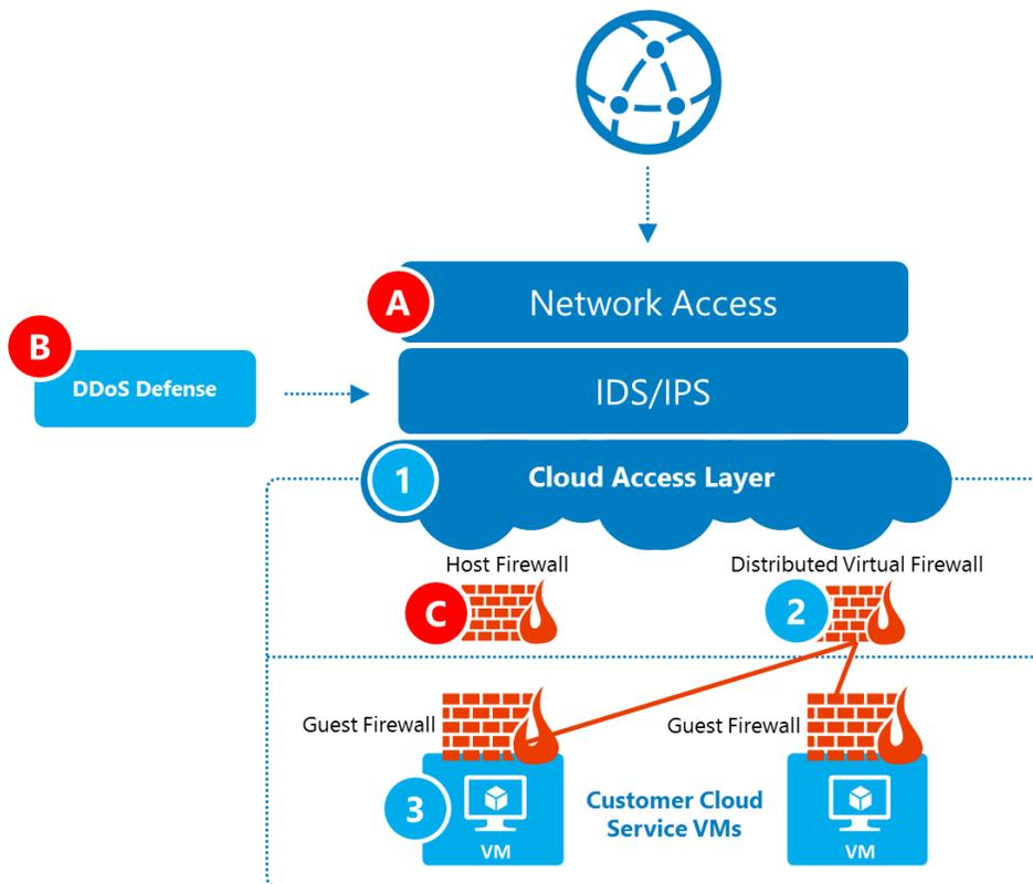
Figure 7. Layers of defense for protecting customers and Azure infrastructure.
