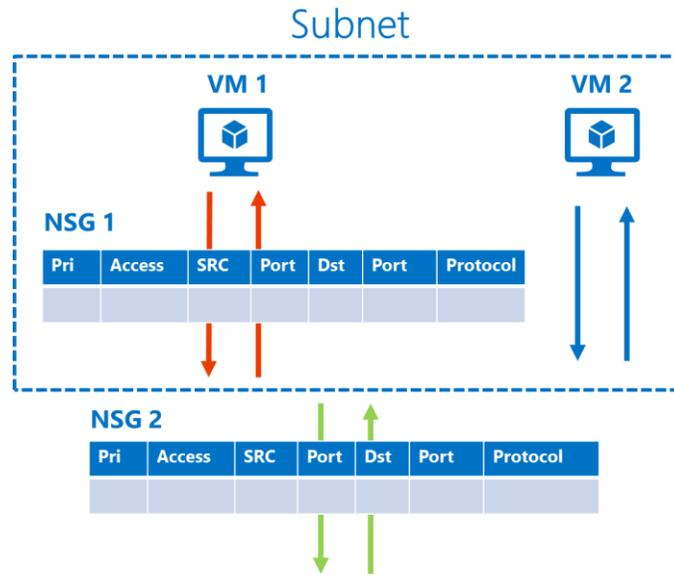
Figure 5: 5-tuple rules processing in a Virtual Network.
