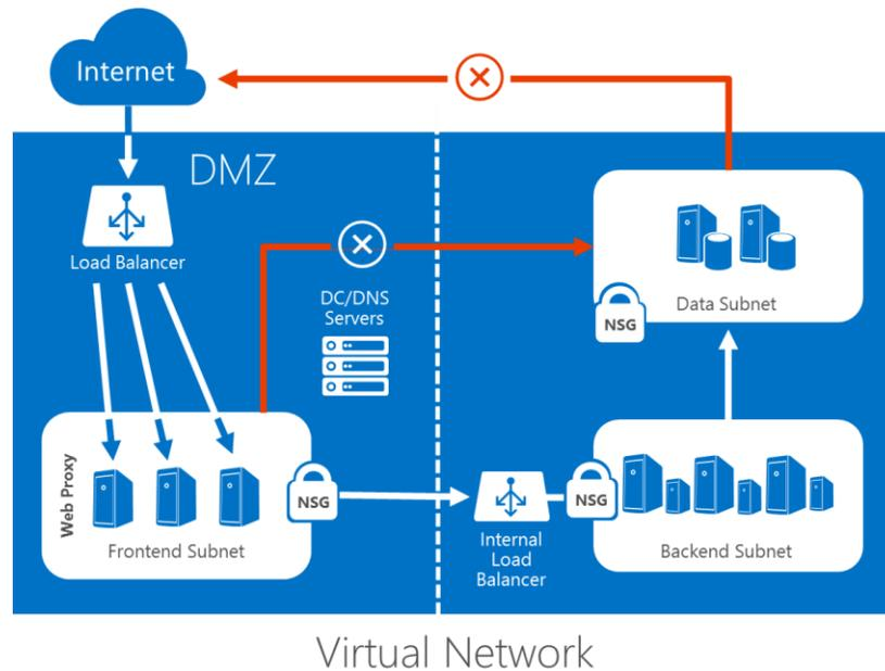
**Figure 4: Using Network Security Groups in a multi-tier application VNET.**
